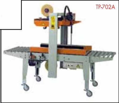
Automatic Random Carton Sealer. Great for running different box sizes.
